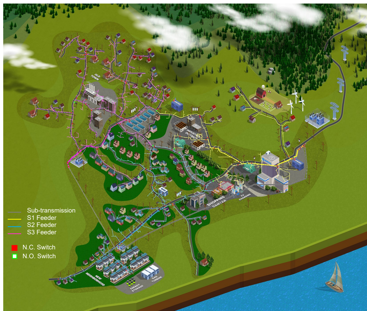
Figure 4: A feeder plot colored by topological isolation illustrating the boundaries of the S1, S2, and S3 sub-feeders overlaid on a semi-geographic view of DERs, rooftop PV, and volt-var control equipment assets.
